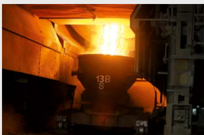
Monitoring of the refractory lining of a slag ladle car while pulling out of the factory
